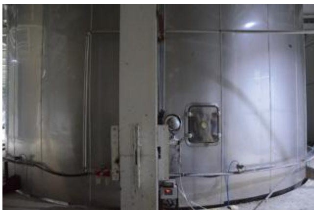
Built-in fluidized bed agglomeration granulation
